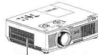
Air Intake Vent
