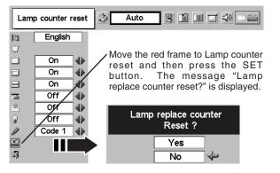
NOTE : Do not reset the Lamp Replace Counter until after the Projection Lamp is replaced.
