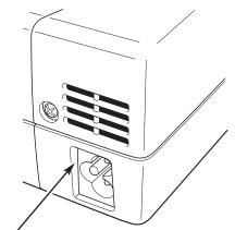
Connect AC Power Cord (supplied) to a projector. The AC outlet must be near this equipment and must be easily accessible.
