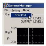
7. In the COM Port Setting dialog, select the COM port from the drop-down list that your projector is connected to.
