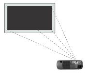
The projector can be off-set vertically or horizontally from the center of the screen and be optically corrected without causing distortion to the image.
