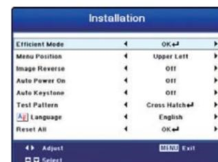
Energy-efficient modes can be set using installation setup screen
