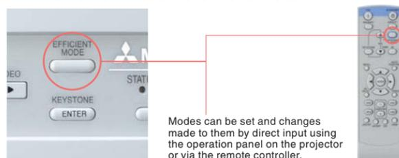
Modes can be set and changes made to them by direct input using the operation panel on the projector or via the remote controller.
