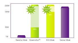
ViewSonic's exclusive DynamicEco™ mode reduces projector brightness to 30% to extend lamp life and lower energy consumption. DynamicEco™ mode will automatically kick in when no signal is present, or can be manually enabled through a button on the remote. It also reduces fan noise to eliminate distractions.
