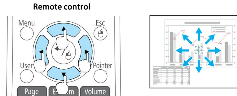
When any pair of adjacent [⬆], [⬇], [⬅], or [➡] buttons are pressed at the same time, the pointer can be moved diagonally.
