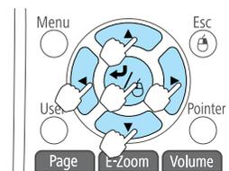
While holding down the [Left Arrow] button, press the [Left Arrow], [Right Arrow], [Up Arrow], or [Down Arrow] button to drag.
