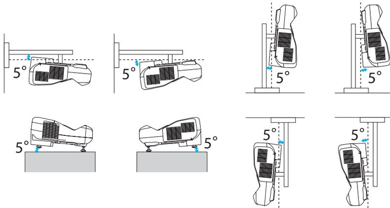
If you use the projector tilted at an angle of more than 5° it could be damaged and cause an accident.
