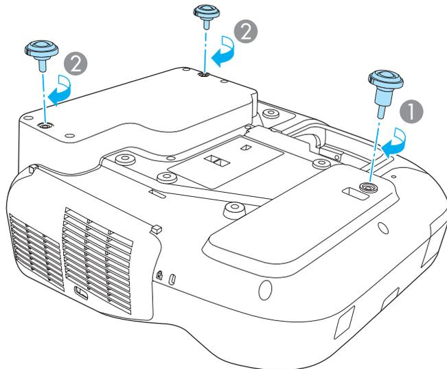
1 Insert the foot with the spacer into the front foot fixing point.
