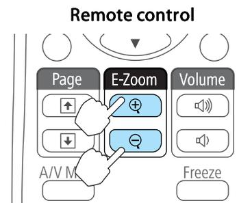
[⊕] button: Expands the area each time it is pressed. You can expand quickly by holding the button down.
