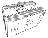
Removing the projector battery:
