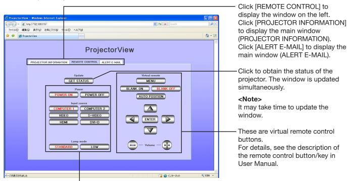
These buttons are used to control the projector's power, input source, and lamp mode.
