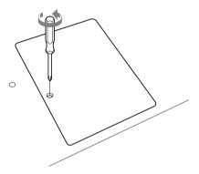
**3** Loosen the 2 screws on the lamp then pull out the lamp by its grab.
