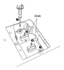
**4** Insert the new lamp all the way in until it is securely in place. Tighten the 2 screws.
