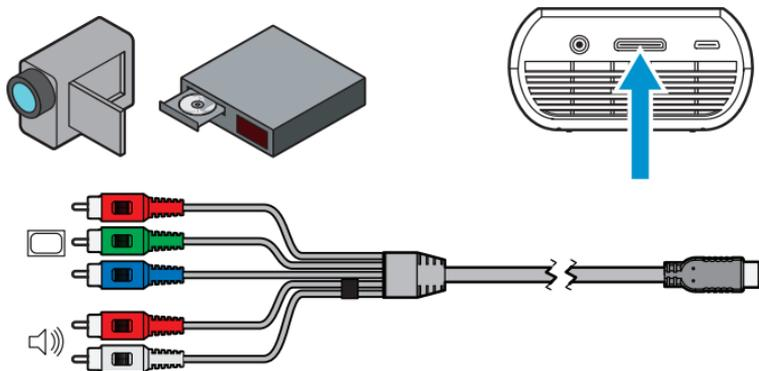
*Important Note: There are two red connectors on the Component AV cable. One is for the right audio channel and the other is for the Pr component video signal. Be careful to connect the red audio to red audio and red video to red video. If these connectors are switched, the projected image will appear green and an abnormal noise will come from the right speaker.*
