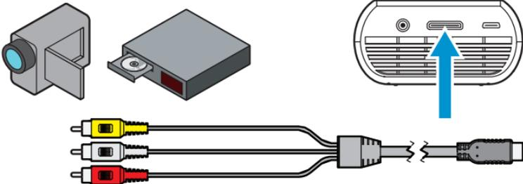
*Tip: Some video devices do not have the standard audio and video connections and may require an AV cable specified by the manufacturer. The AV cable allows you to connect your video device to your TV monitor or your projector and may be purchased from the video device manufacturer. Once you have the AV cable, use the cable adapters to connect the video device cable and the projector cable.*
