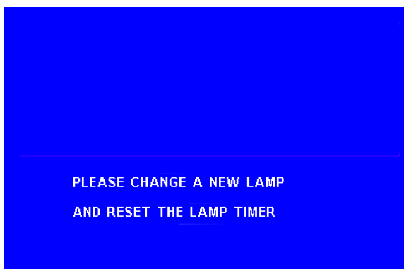
Figure 15 Lamp replacement warning signal
