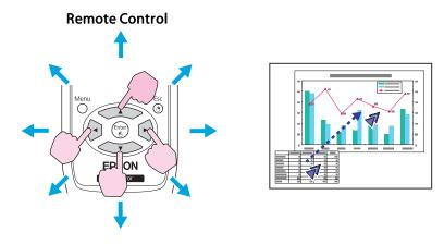
When pressed in conjunction with the adjacent [ ], [ ], and [ ] buttons, the pointer can be moved diagonally.
