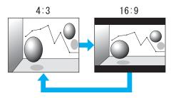
\* When a 720p/1080i signal is input, the display is in a zoomed 4:3 format (the image is cut off on the right and left sides).
