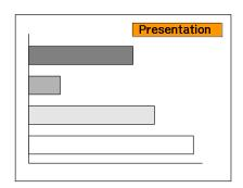
Each time you press the button, the Color Mode name is displayed on the screen and the Color Mode changes.
