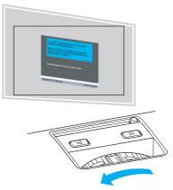
If the projected area is still not larger than the frame even after adjusting the Zoom ring to its maximum size, try moving the projector further away from the screen. (If this causes the message box moves away from the center of the screen, adjust it so that it is centered again.)
