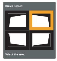
Using the [ ], [ ], [ ], and [ ] buttons on the remote control, or the [ ], [ ], [ ], and [ ] buttons on the control panel, correct the position of the corner.
