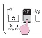
When the following message box appears, move the projector to adjust the position of the projected image, so that the message box is at the center of the screen.
