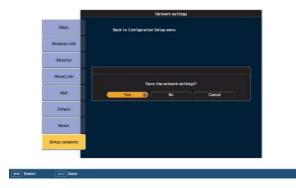
This completes the setup of the connection between the projector and the access point. Press the [Menu] button to close the Configuration Menu.
