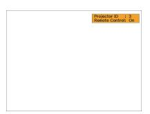
When you press the buttons, the current Projector ID is displayed on the projection screen. It disappears in about three seconds.
