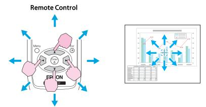
When pressed in conjunction with the adjacent [ ], [ ], and [ ] buttons, the pointer can be moved diagonally.
