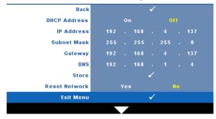
**DHCP ADDRESS**—If a DHCP server exists in the network to which the projector is connected, the IP address will automatically be acquired when you select DHCP On. If DHCP is Off, manually set the IP Address, Subnet Mask, and Gateway. Use to select the number of IP Address, Subnet Mask, and Gateway. Key in Enter to confirm each number and then use \( \) to set the next item.
