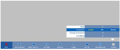
**e** Enabling the Password function will pop up a character screen, key in a 4-digit number from the screen and press .
