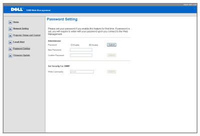
Use Password Setting to set up an administrator password to access the **Web Management**. When enabling password for the first time, set the password before enabling it. When the password function is enabled, the administrator password will be required for accessing the **Web Management**.
