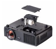
9 Reset the lamp usage time by selecting "Yes" for Lamp Reset in the OSD Lamp tab (see Lamp menu on page 39). When a new lamp module has been changed, the projector will automatically detect and reset the lamp hours.
