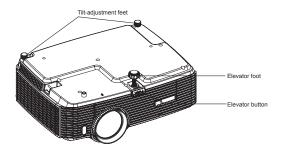
The projector is equipped with an elevator foot to adjust the image height. To raise or lower the image:
