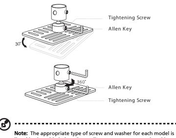
**Note:** The appropriate type of screw and washer for each model is listed in the table below. 3 mm diameter screws are enclosed in the screw pack.
