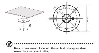
2 Secure the ceiling rod using the appropriate type of four-cylinder screws.
