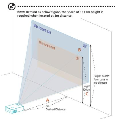
Figure: Fixed distance with different zoom and screen size.
