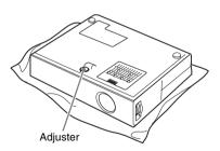
2 Slide switch A in the slit in front of the adjuster in the direction of the arrow (toward the front panel of the projector) with the small minus screwdriver. The lens protector and the tilt adjuster are switched to the emergency mode.
