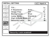
**5** Turn the main power off and disconnect the AC power cord. The security lock is set to on, then it becomes effective. The screen for entering the password is displayed when the power is turned on the next time.
