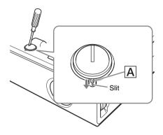
**3** When opening/closing the lens protector, turn the groove of the adjuster with a coin.
