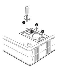
**4** Insert the new lamp all the way in until it is securely in place. Tighten the screws. Fold the handle.
