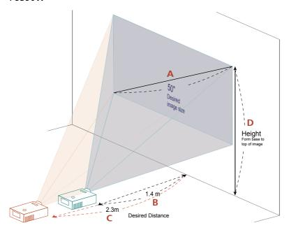
The table below shows how to achieve a desired image size by adjusting either the position or the zoom ring. For example: to obtain an image size of 50" set the projector at a distance 1.4 m and 2.3 m from the screen and adjust the zoom level accordingly.
