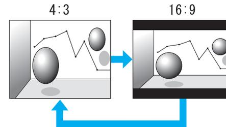
\* When a 720p/1080i signal is input, the display is in a zoomed 4:3 format (the image is cut off on the right and left sides).
