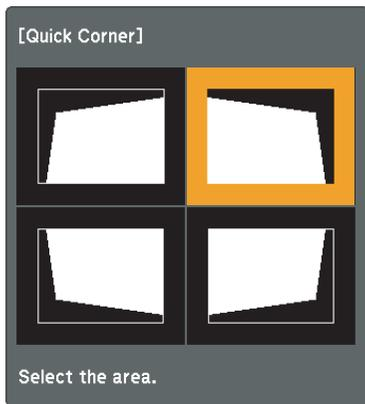
**4** Using the [↖], [↗], [↙], and [↘] buttons on the remote control, or the [↖], [↗], [↙] and [↘] buttons on the control panel, correct the position of the corner.
