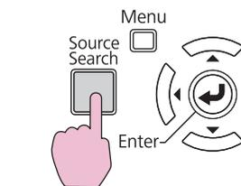
When two or more pieces of equipment are connected, press the [Source Search] button until the target image is projected.
