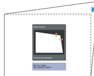
If the triangle in the direction you are adjusting the shape turns gray, as shown in the screenshot below, you cannot adjust the shape any further in that direction.
