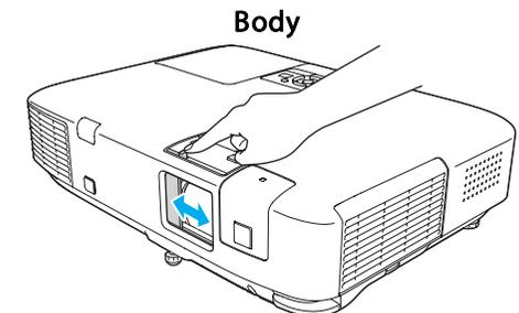
Each time you press the button, or open/close the lens cover A/V Mute turns on or off.
