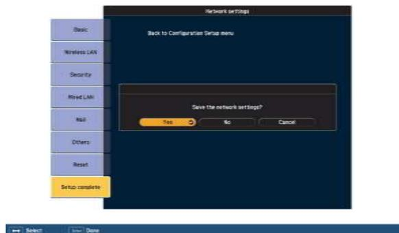
This completes the setup of the connection between the projector and the access point. Press the [Menu] button to close the Configuration Menu.
