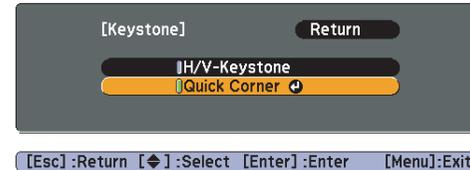
Press the [Enter] button again to display the selection screen from which you can select one of the four corners.
