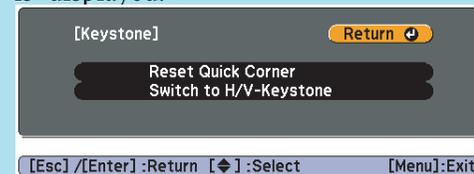
**Reset Quick Corner:** Resets the result of Quick Corner corrections.
