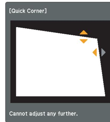
**5** Repeat procedures 3 and 4 as needed to adjust any remaining corners.
