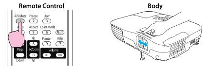
Each time you press the button, or open/close the lens cover A/V Mute turns on or off.
