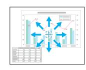
When pressed in conjunction with the adjacent [] $[(\bullet)][(\bullet)]$  buttons, the pointer can be moved diagonally.
