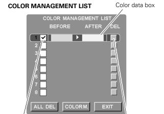
Clear the check mark if you do not want to apply this adjusted color data to the projected image. Select the DEL box if you want to delete the adjusted data. A confirmation box appears.
