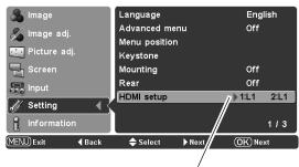
Press the Point ▶ or OK buttons to select L1 or L2 according to the output signal of video equipment.
