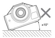
Avoid tilting the projector more than  $\pm$  10 degrees, and avoid installing it in place other than a floor. Doing so may cause color shading or shorten the lamp life excessively.
