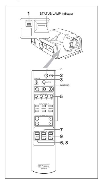
1 Set the main power switch on the left side of the projector to the upper position.
