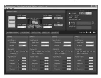
**3** Click any of the PICTURE CONTROL, COLOR/FRAME and INSTALLATION buttons to display the desired control window.
