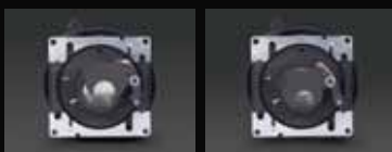
Fully open iris (2700:1) Stopped down iris (4000:1)
