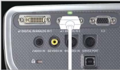
LED indicates connector responding to image signal.
