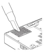
When it becomes difficult to remove the dust from the filter with a vacuum cleaner, remove the air filter and wash it.
