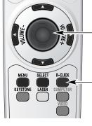
\_PRESENTATION POINTER button Move the pointer on the screen with this button.
