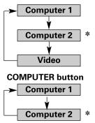
Computer 2 is not displayed when the COMPUTER IN 2/COMPONENT IN/MONITOR OUT terminal is used as Monitor out.
