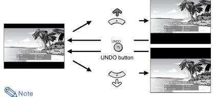
Press ▲ to move the projected image upwards.
