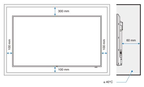
**NOTE:** The maximum environmental operating temperature of the monitor is 40 °C. This monitor has internal temperature sensors.
