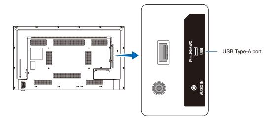
NOTE: • Check the connector shape and orientation when connecting the USB device or cable.
