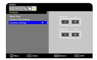
a. Press the OK button of the remote control. Place the cursor on [Power On] and press the OK button of the remote control to enable the [Power On]. Press the ◀, ▶ buttons of the remote control to move between the hours and minutes fields.
