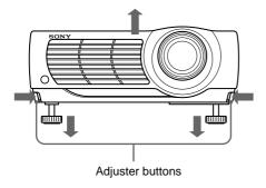
**2** While pressing the buttons, adjust the height. Then, release the buttons.
