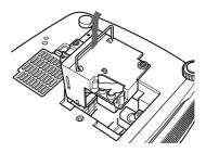
**5** Insert the new lamp all the way in until it is securely in place. Tighten the two screws. Fold down the handle.
