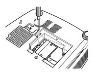
**4** While holding the handle and keeping the lamp unit horizontal, pull straight up.
