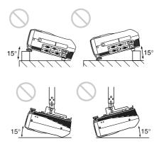
Avoid tilting the unit at an angle of more than 15 degrees. Installation of the unit in this manner may cause a malfunction.
