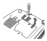
**3** Loosen the screws on the lamp unit with the Phillips screwdriver.
