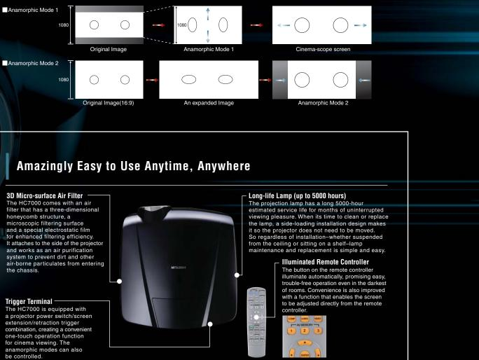
filter that has a three-dimensional honeycomb structure, a microscopic filtering surface and a special electrostatic film for enhanced filtering efficiency. It attaches to the side of the projecto and works as an air purification system to prevent dirt and other air-borne particulates from enterin the chassis.
