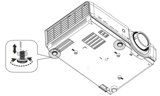
To adjust the angle of the picture, turn the Adjustable feet right or left until the desired angle has been achieved.
