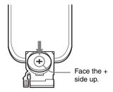
**3** Put the lithium battery holder back into the Remote Commander.
