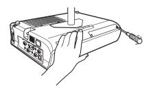
**3** Place your fingers under the lamp cover and pull it up to remove the lamp cover.
