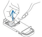
(2) Vacuum off accumulated dust and dirt on inside and outside of the filter case.
