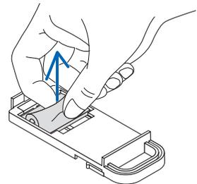
(2) Vacuum off accumulated dust and dirt on inside and outside of the filter case.
