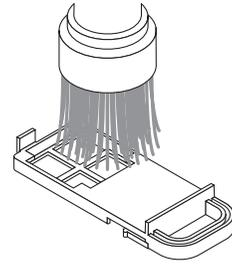
(3) Fix a new Filter (B) onto the filter case.
