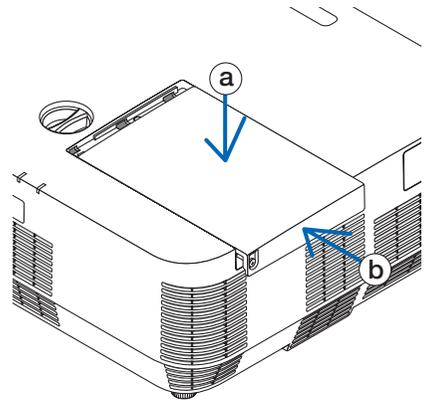
(2) Tighten the screw to secure the lamp cover.
