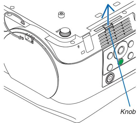
**3. Remove the Filter (A) from the filter case.**
