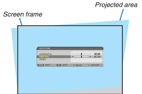
3. Align the left (or right) side of the screen with the left (or right) side of the projected image.
