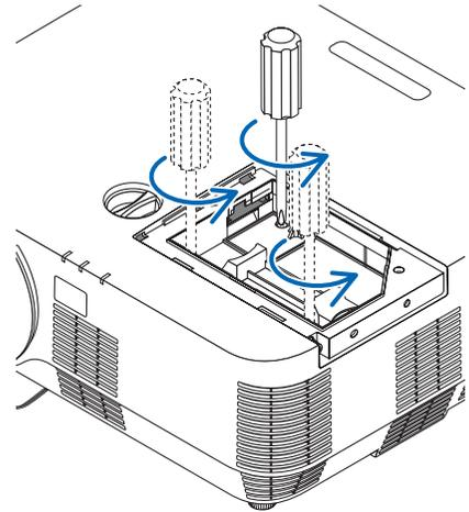
(2) Remove the lamp housing by holding it.
