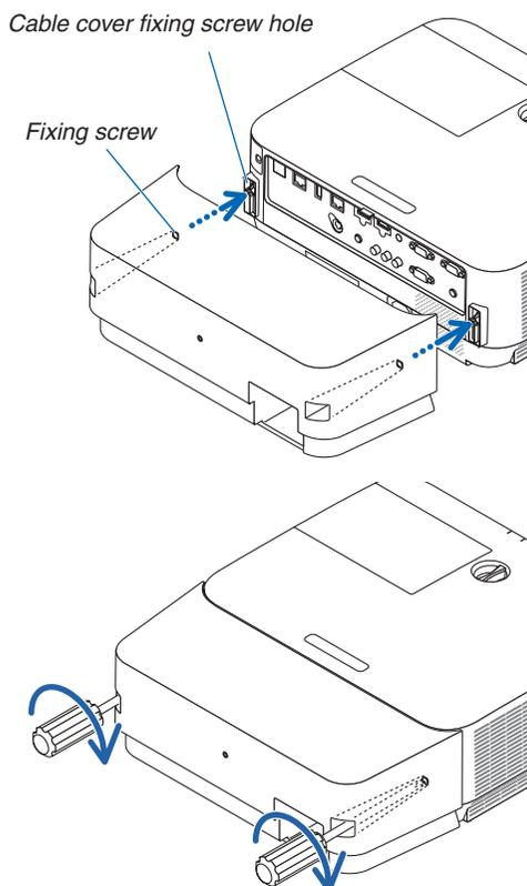
**Removing the cable cover**
