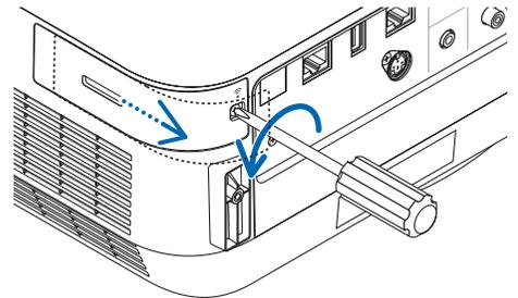
3. Insert the wireless LAN unit into the USB (wireless LAN) port.
