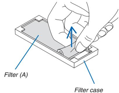
**3. Vacuum all the dust on inside and outside of the filter case.**
