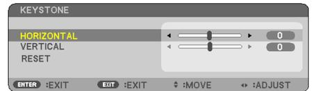
2. Press the ▼ button to select [VERTICAL] and then use the ◀ or ▶ so that the left and right sides of the projected image are parallel.
