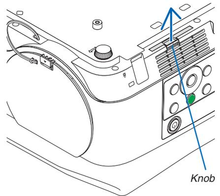
**2. Remove the Filter (A) from the filter case.**
