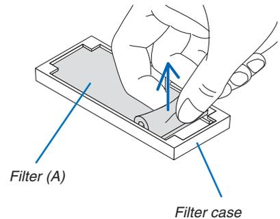
**4. Vacuum all the dust on the Filter (A) and the filter case.**
