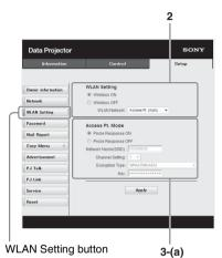
Enable or disable the radio wave output of USB wireless LAN module.
