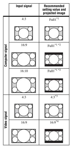
\*1: If you select "Normal," the image is projected in the same resolution as the input signal without changing the aspect ratio of the original image.
