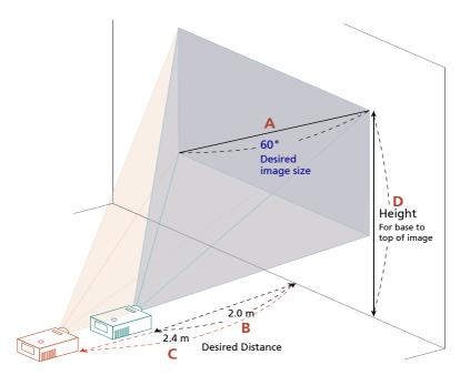
The table below shows how to achieve a desired image size by adjusting either the position or the zoom ring. For example: to obtain an image size of 60" set the projector at a distance 2.0 m and 2.4 m from the screen and adjust the zoom level accordingly.
