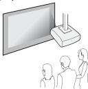
• Suspend the projector from the ceiling and project images from behind a translucent screen. (Rear/Ceiling projection)
