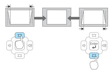
Press the [4] or [4] buttons to correct horizontal distortion.
