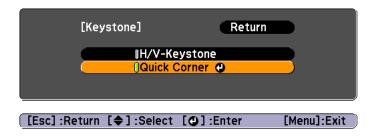
Using the [ ], [ ], and [ ] buttons on the remote control, or the [ ], [ ], and [ ] buttons on the control panel, select the corner to correct, and then press the [ ] button.
