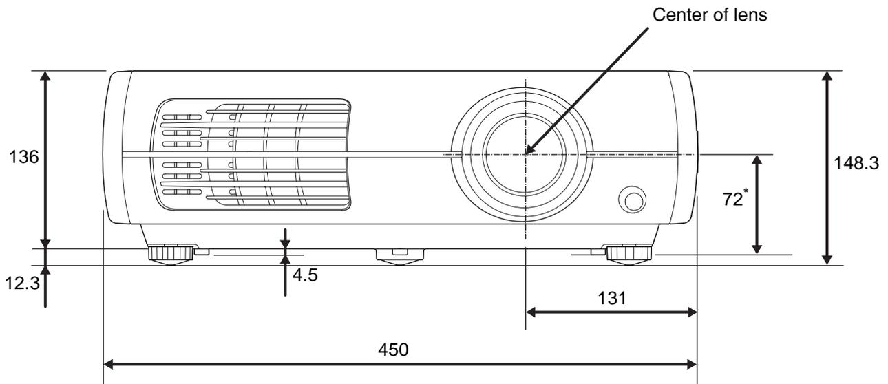
\* Distance from center of lens to suspension bracket fixing point
