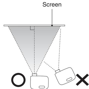
Set up so that the projector is parallel to the screen. If the projector is set up at an angle to the screen, distortion of the images will occur.
