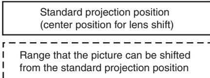
**Attention** When transporting the projector, make sure to turn the lens position down by the full amount. Otherwise the lens shift mechanism may be damaged.
