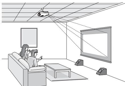
\* If you place the projector off to the side, aim it straight ahead (rather than at the center of the screen), then use the horizontal lens shift dial to center the image on the screen.
