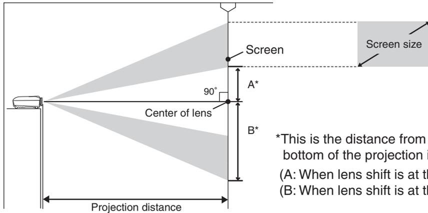
\*This is the distance from the center of the lens to the bottom of the projection images.
